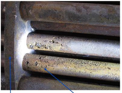
Baffle plate w/o signs of corrosion pits
