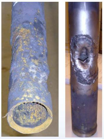
Example of boiler tube failier
