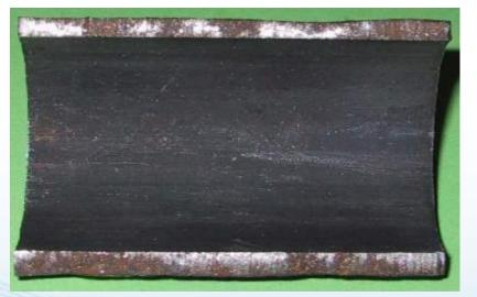
Magnetite Layer in Water-Tube Boiler
