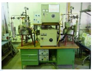
Shell boiler simulation at university of Rostock at "steady state" conditions, p = 15 bar
