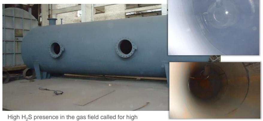
High H<sub>2</sub>S presence in the gas field called for high performance corrosion protection to 32 new build carbon steel vessels.
