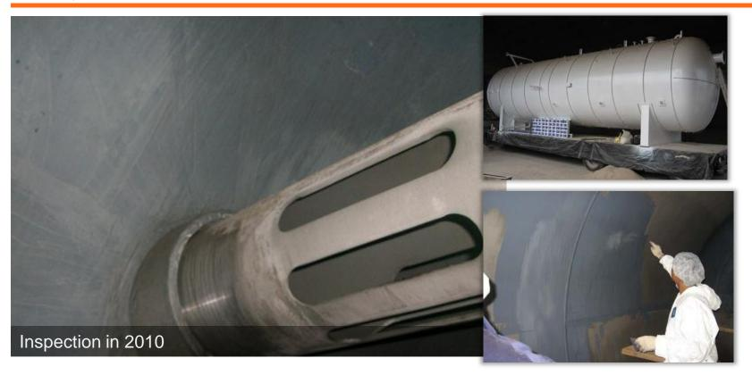
Flash drum to be exposed to diglycolamine, wet H<sub>2</sub>S and CO<sub>2</sub> at 80°C.
