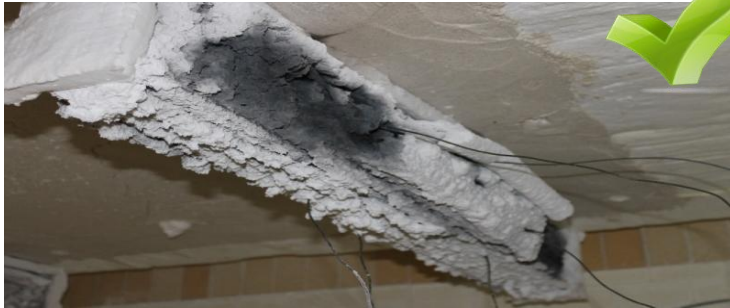
Good stickability steel-primer and primer-intumescent
