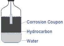
Coupon Wt. Loss, Good for Low Velocity & Temperature; Simple
