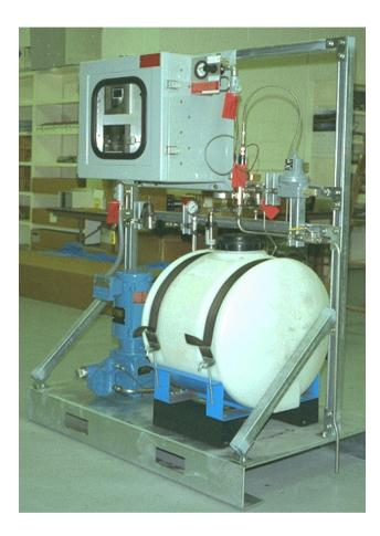
Electrical Resistance (ER) Probes Coupons VTCP (Variable Temp Corrosion Probe) COLA (Condensate On-Line Monitor) • Simulates Dewpoint Continuous pH
