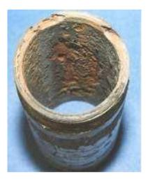
Fe(OH)3 is insoluble leading to an increased corrosion rate as more iron is leached out from the metal to maintain the chemical equilibrium.
