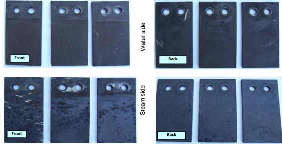
Carbon steel coupons after exposure in water drum under Carbohydrazide dosing boiler #81
