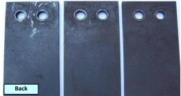
Cupronickel coupons after exposure in HP heater under Carbohydrazide dosing boiler #81
