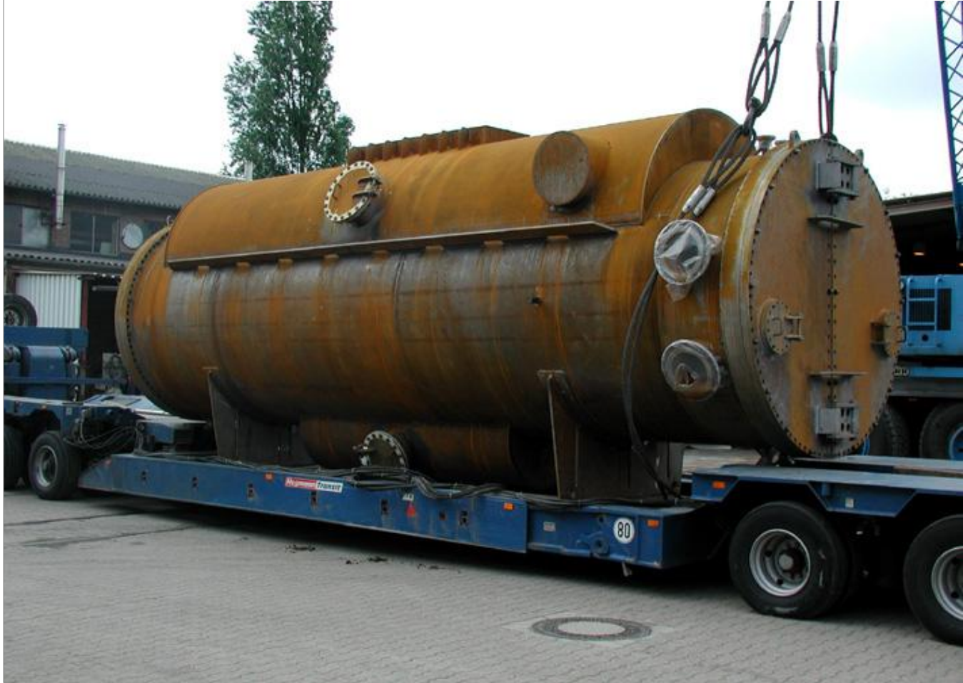
condenser for power plant (ordered by Siemens AG; before coated)
