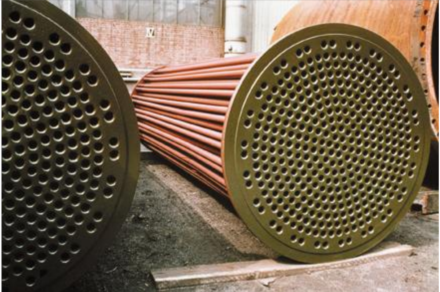
some tube bundles (shell- and tube-side coated)
