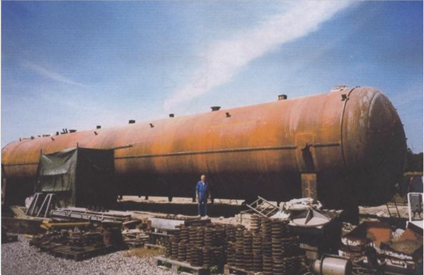
heat cured coating Si 14E of a storage tank
