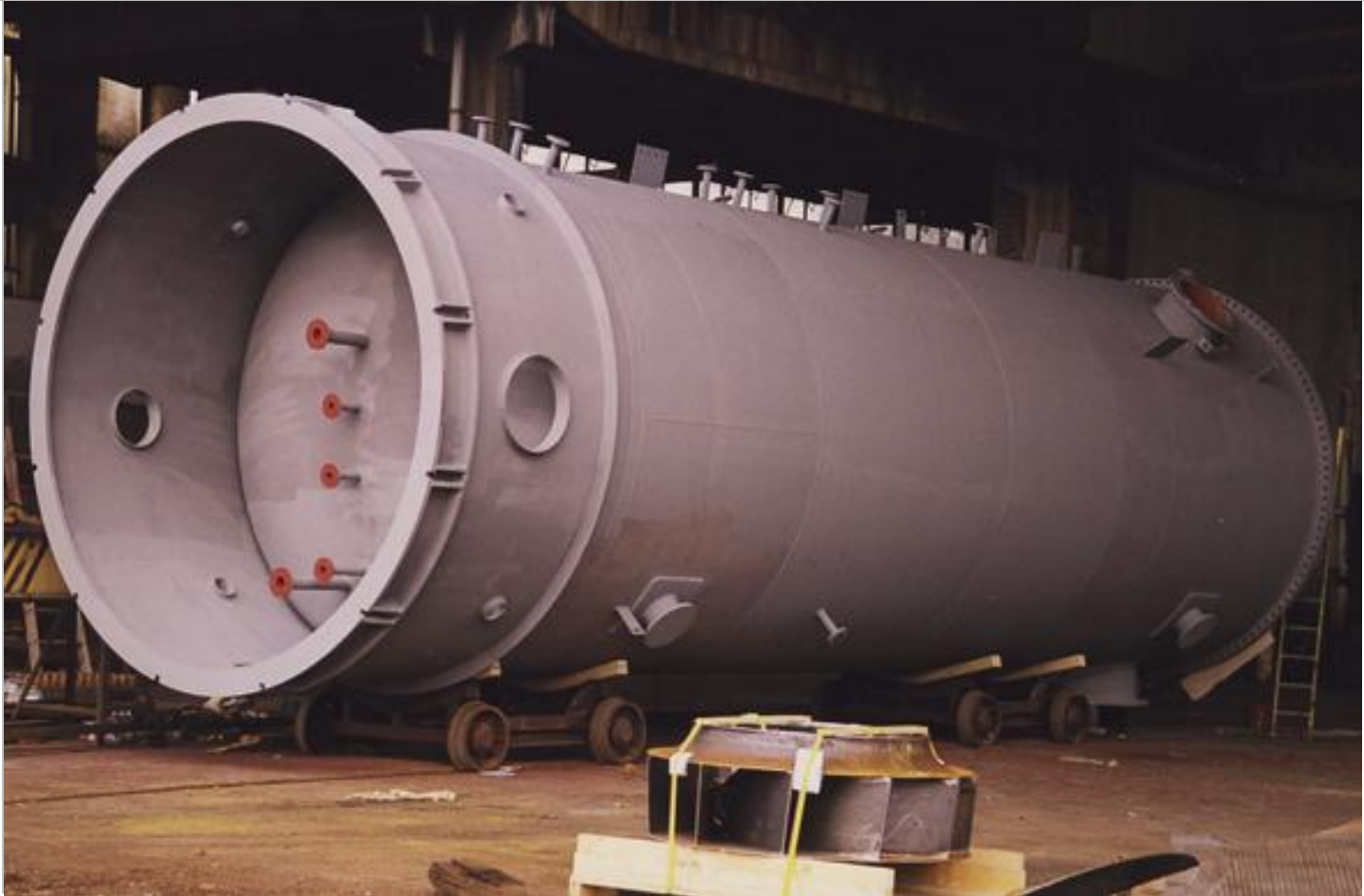
internal heat cured coating Si 14E of a channel
