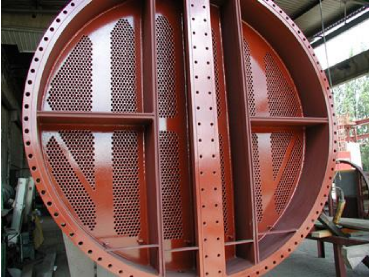
condenser after tube-side coating
