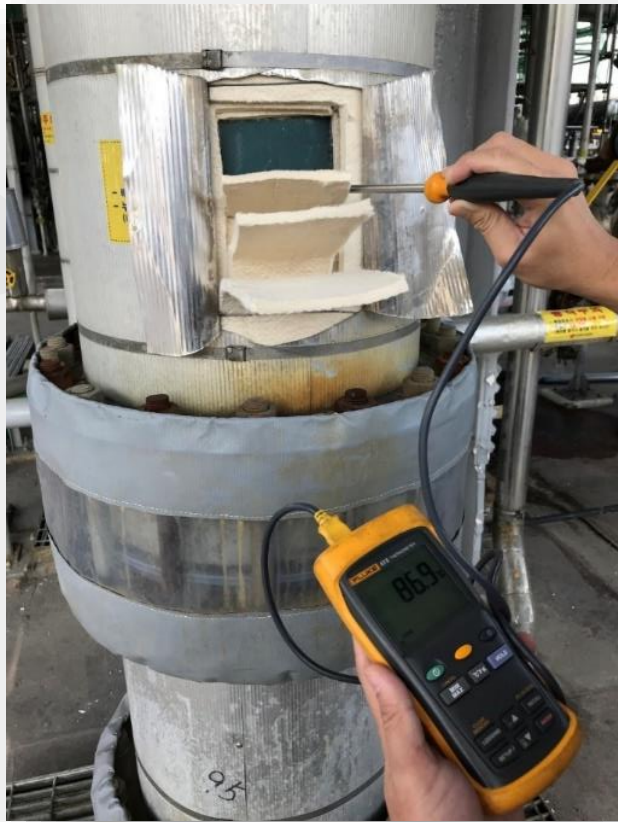
Insulated with 20mm Pyrogel XT
