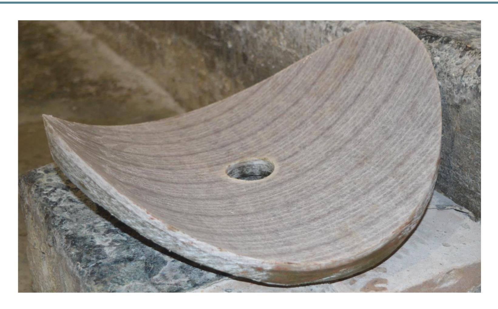
Coupon Cut piece after Hot tapping from the Parent Pipe.
